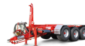
THL 30 (31-34 t total weight, 30 t lifting capacity)
