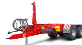
THL 20 (20-24 t total weight, 17-21 t lifting capacity)
