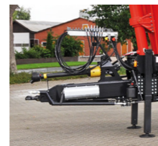
Height-adjustable draw gear with rubber bearing
